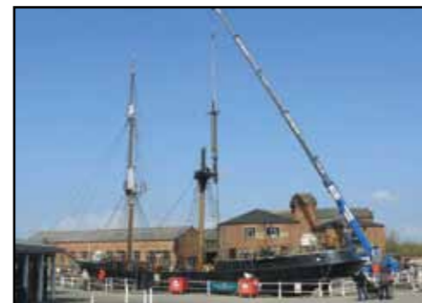
Lifting the main top mast from Kaskelot in the large dry dock. (picture courtesy of Hugh Conway-Jones)
